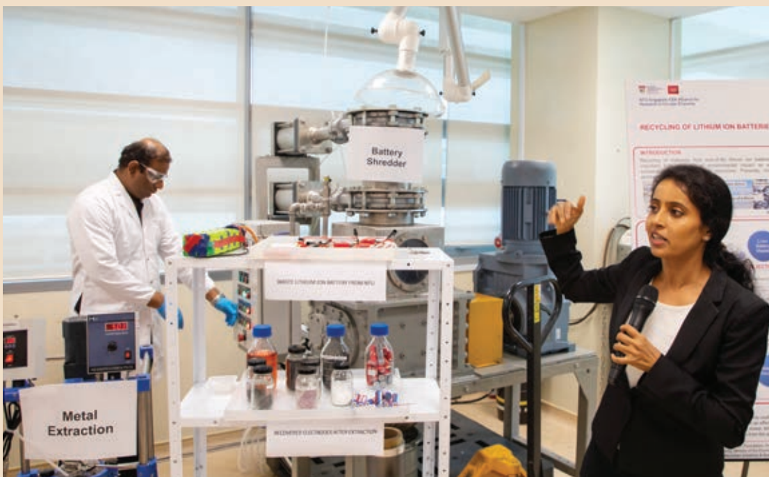
Professor Madhavi Srinivasan, co-director of SCARCE, explains how a battery shredder is used for shredding used lithium ion batteries (LIBs) as an initial step to extract the electrode materials, which can then be reused to produce new LIBs
